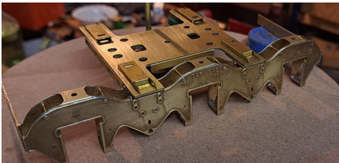
Carel Janse van Rensburg's parts for a EW tender bogie in Cape Gauge 1, 1:24 scale. These tenders were used on the SAR class 23 steam engines, and later on the 15F engines, for which these are destined.
