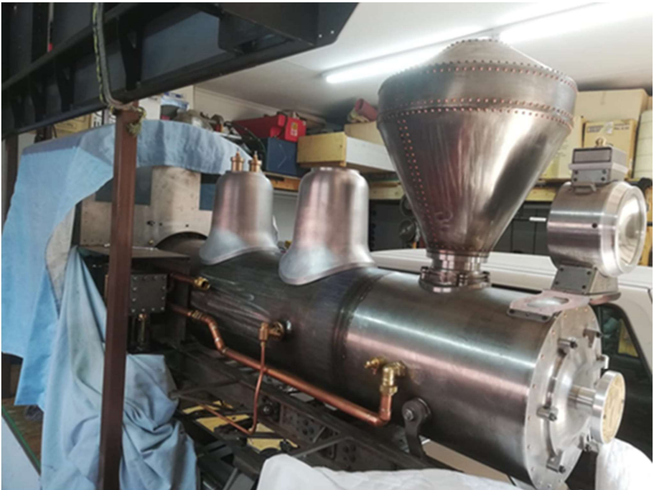
Johnny Sharpe machined and sanded the massive domes on his 7 ¼ inch Shay.
