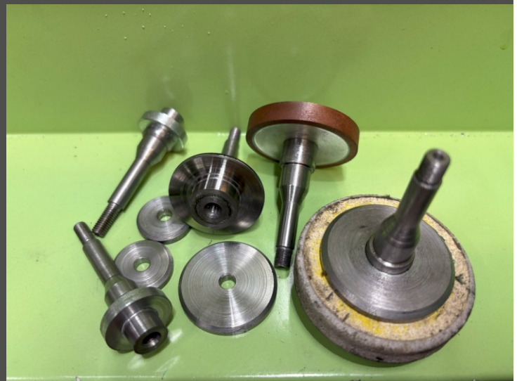
A few extra arbors for Quorn and tool post grinder (above) Fitting a taper lock in a small pulley for a milling slide. (left)
