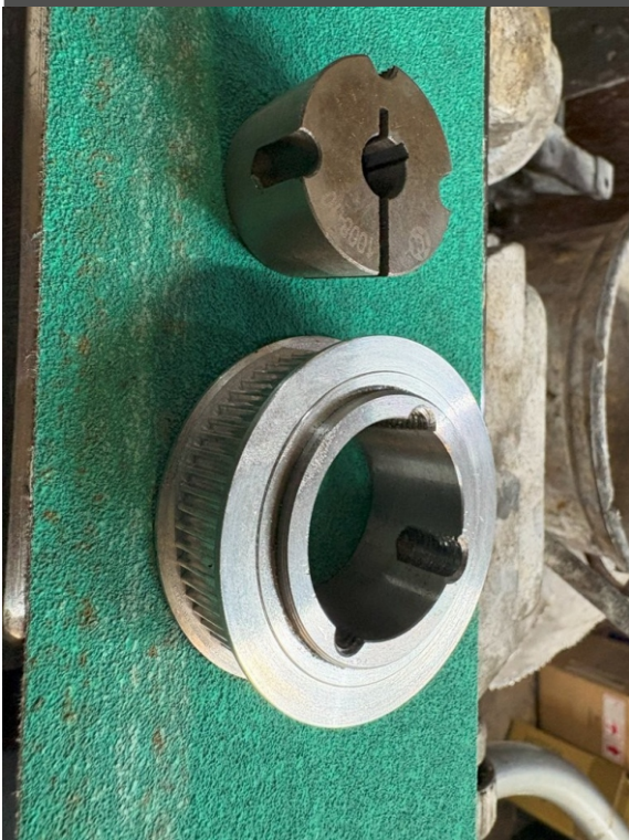
A few extra arbors for Quorn and tool post grinder (above) Fitting a taper lock in a small pulley for a milling slide. (left)
