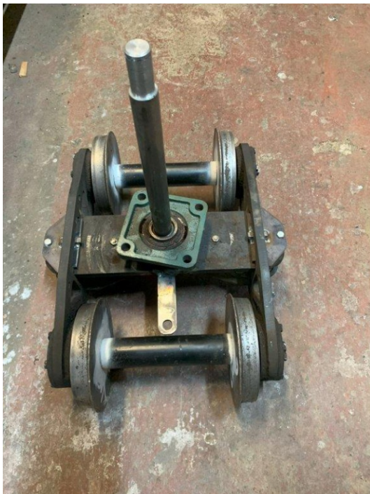
Modified truck bogie for side control on the Dzs, with painted laser cut parts for the conversions.
