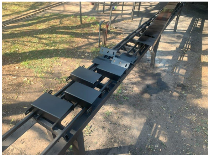
Modified truck bogie for side control on the Dzs, with painted laser cut parts for the conversions.
