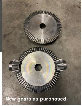
I cut out the centre of the final drive gear and mounted the pinions. The centre boss acts as a spacer and allows the "crownwheel" to rotate on the axle. Silver steel pinion gear shafts. The back bevel gear is fixed to the axle.
