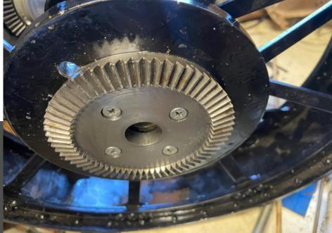
The other bevel gear is mounted directly on the near wheel which freewheels on the axle.
