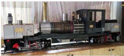
John always wanted to build a Shay and acquired a set of drawings of Ron Etters' Siver City Shay, but proceeded to redesign and scale up the whole locomotive. He converted it from a 2 truck to a 3 truck locomotive and within two and a half years Lady Shay was born.
