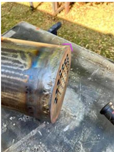
Tube plate welded nicely
