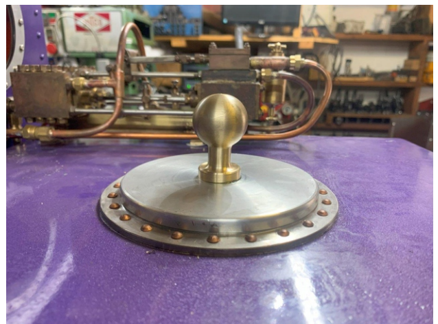
Fan repairs, Theresa oils from Stainless square tubing for the tank with floor welded on. One of Theresa filler lid, could not resist the brass handle knob. By Leon Kamffer.
