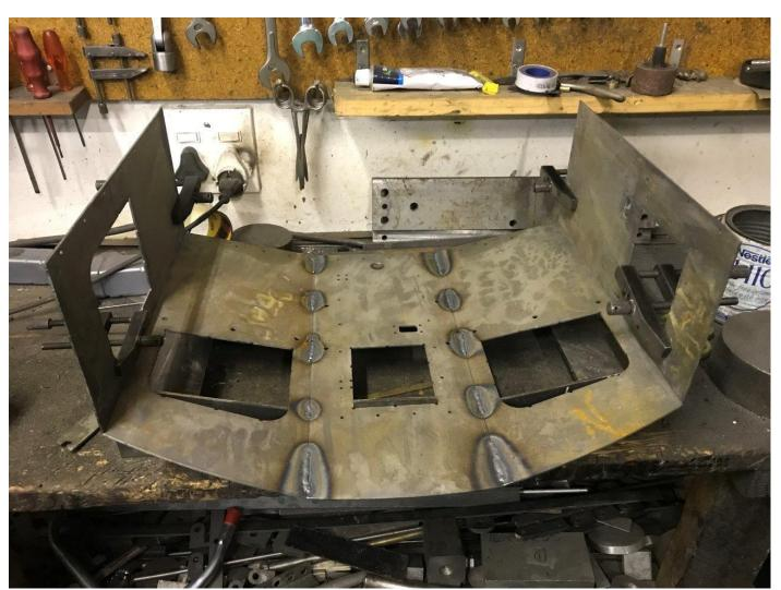
Foto showing cab assemblies in jig to weld them.
