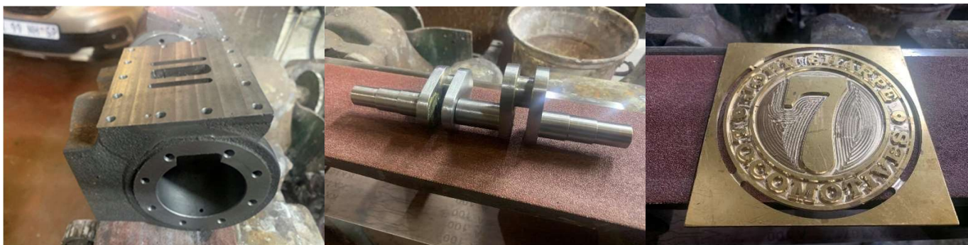
Cylinder for Bagnall "Teresa" crank axle for Neil's Midland engraving for John Sharpe's Shay
