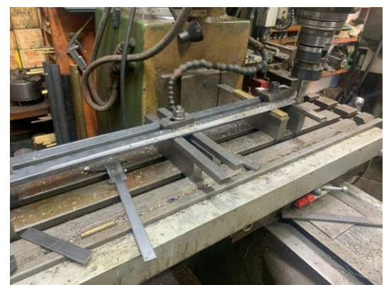
Milling the tracks for the 5 inch crossover for the modified track section.
